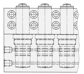
Double-acting threaded-body cylinders as pulltype cylinder for a multiple clamping fixture to mill a wrench flat
